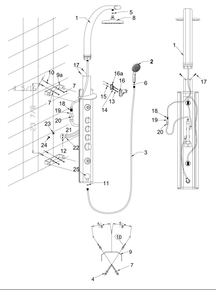
Refer to the technical diagram to choose the proper location for your shower column. You can adjust the column's vertical position based on the person's height. Measurements given in the technical diagram are based on the average human height ( $68^{\circ} - 70^{\circ}$ ).
