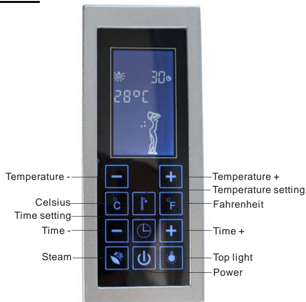
Function Illustration of the Control Board
